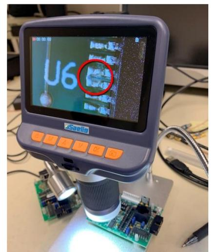
FIG.3 SOLDER BRIDGE SHORT CIRCUIT REVEALED ON MICROSCOPE
