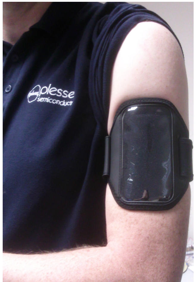
Figure 9 –Sports Armband in position. Sensors are in contact with the underside of the arm, adjacent to the armpit
