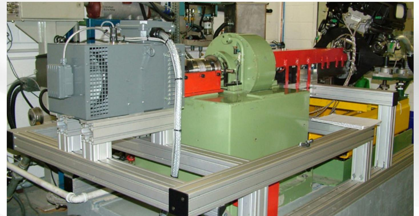
A precision torque sensor actually allows a design engineer to measure torque change at the exact moment when a drive is ideally switched from power to regeneration, to make the most of the falling load potential energy release.
