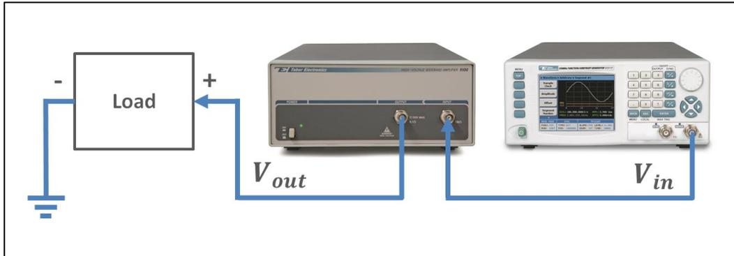
Figure 7: Tabor's Signal source + amplifier driving a load
