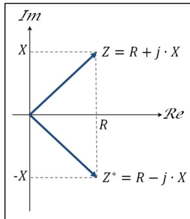
Figure 1: Source & load impedance are complex-conjugates.
