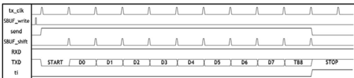
Figure 6.9 Timing Diagram for UART Transmission Mode2
