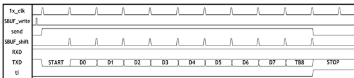
Figure 6.10 Timing Diagram for UART Transmission Mode3
