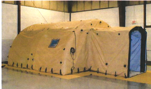
Figure 1: 15' by 20' EMI/RFI airframe enclosure with external foyer.
