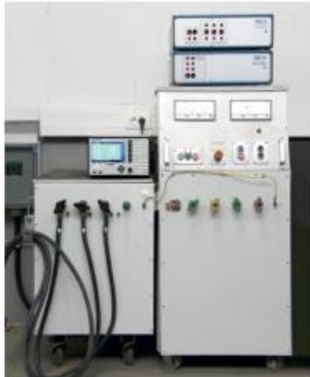
Figure 4: Conventional testing system up to 500A with variable transformer, top right the Power Choke Tester DPG10-4000B/F with 3-Phase Extension Unit in comparison
