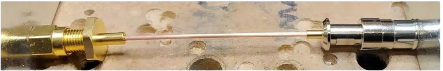
Figure 7 – The test cable in situ, ready to make the TDR measurement.
