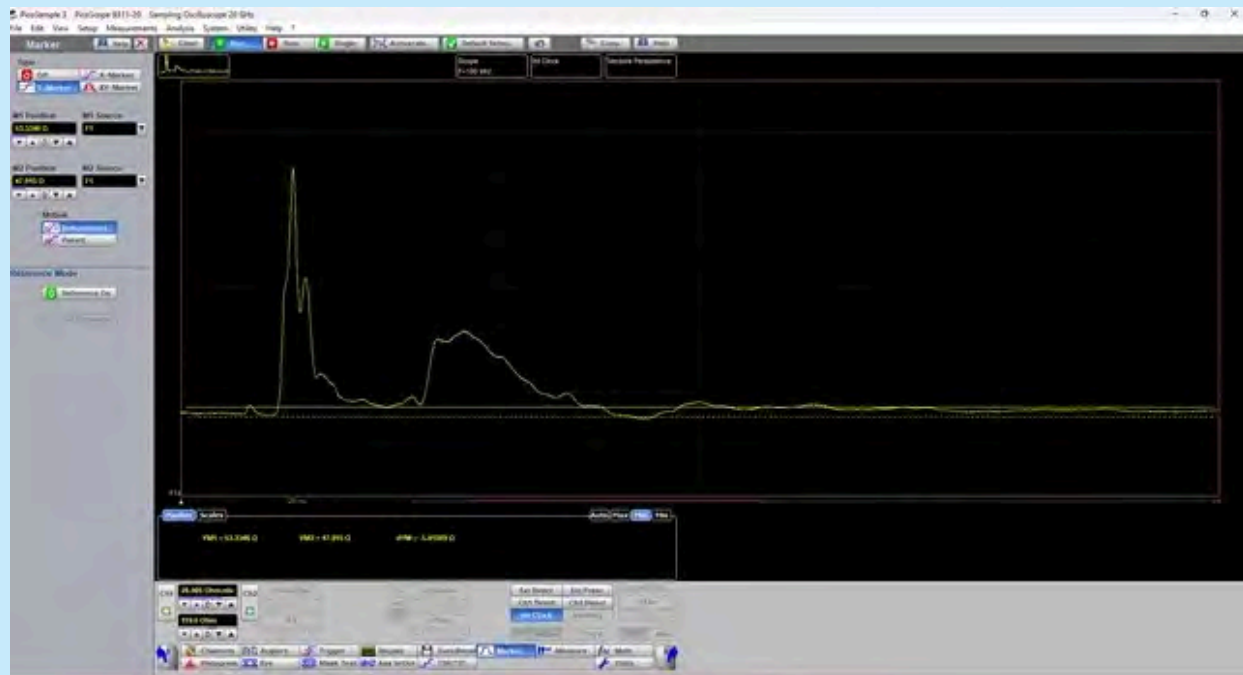
Figure 1 – TDR test results with the cable connected. Pin 49 yellow/grey to blue/black grounding, terminated to 50 \Omega .
