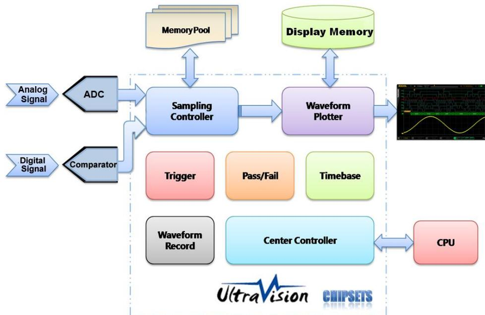
Another extremely important part of the **UltraVision** chipset is the huge data memory. With this it is possible to maintain the maximum sampling rate especially on longer Time/Division settings. This is very important if there is a need to acquire signals over longer time periods, but without losing any signal details.
