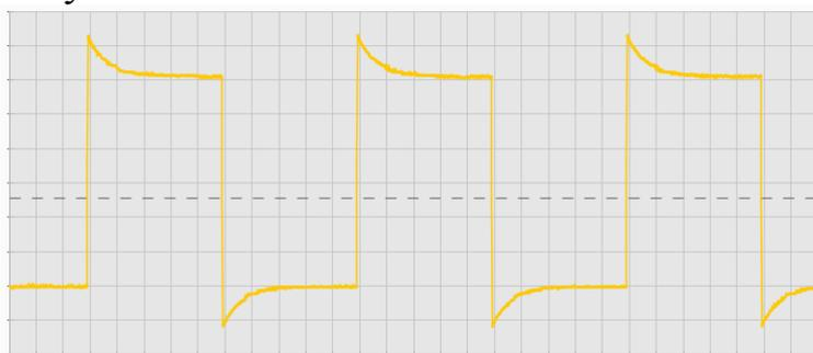
6. You may find you need to connect the ground clip to either the BNC ground or use the GND pad near the compensation output<sup>11</sup> to achieve a clean waveform with minimal mains “hum”
